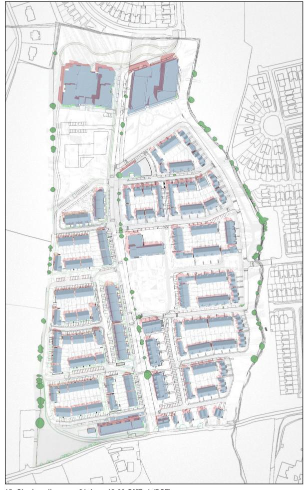
Figure 15: Shadow diagrams 21 June 12:00 GMT+1 (DST)
