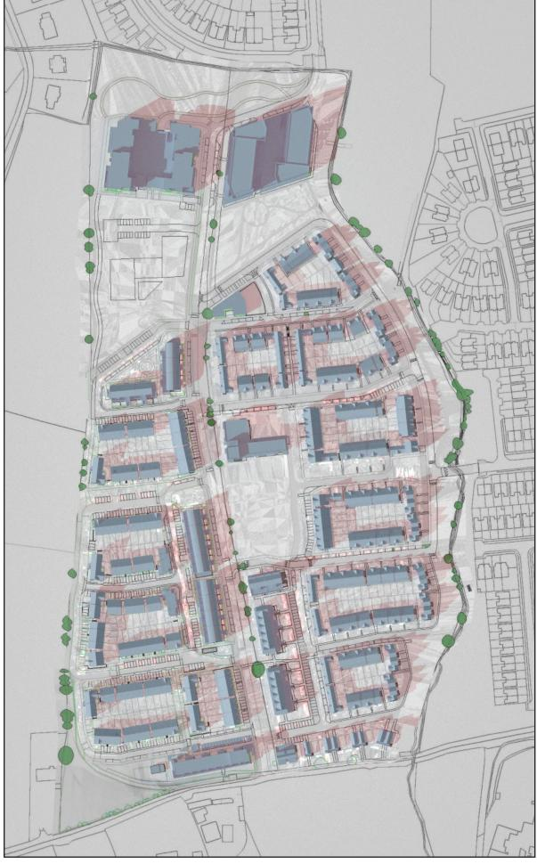
Figure 23: Shadow diagrams 21 September 17:00 GMT+1 (DST)
