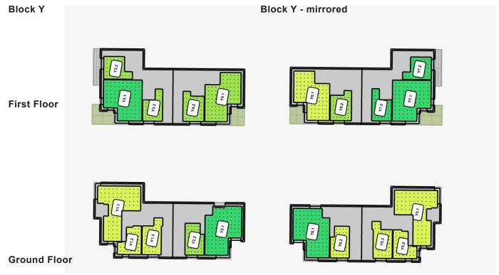
Figure 67: Block Y & Y mirrored - Daylight Provision
