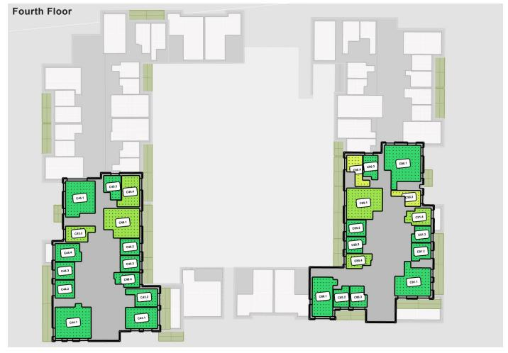
Figure 57: Block C - Fourth Floor Daylight Provision
