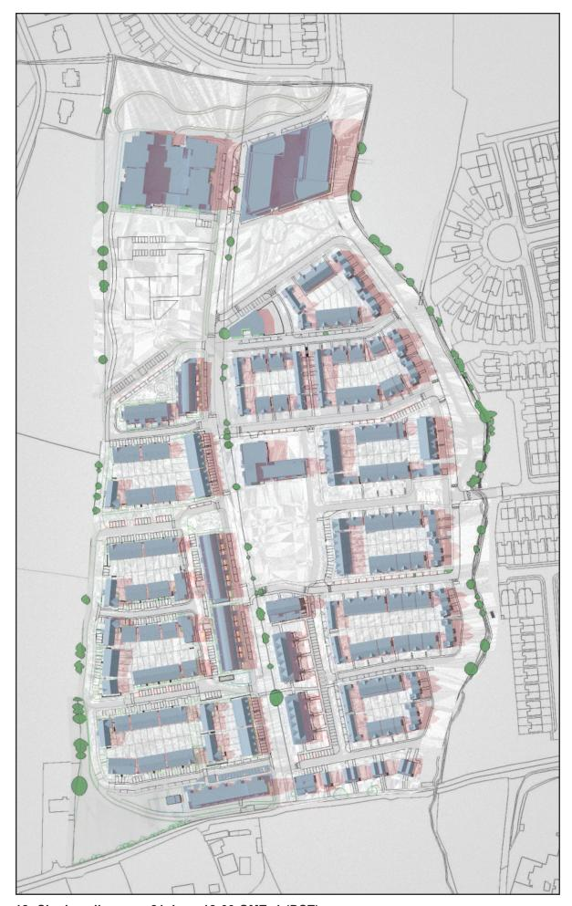
Figure 18: Shadow diagrams 21 June 18:00 GMT+1 (DST)
