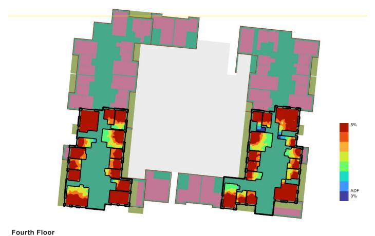
Figure 37: Block C - Fourth floor false colour plan of ADF. Scale 0 - 5%
