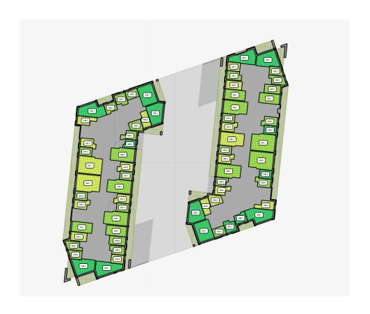
Figure 49: Block A - Second Floor Daylight Provision
