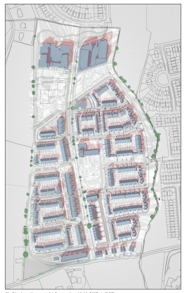
Figure 22: Shadow diagrams 21 September 15:00 GMT+1 (DST)
